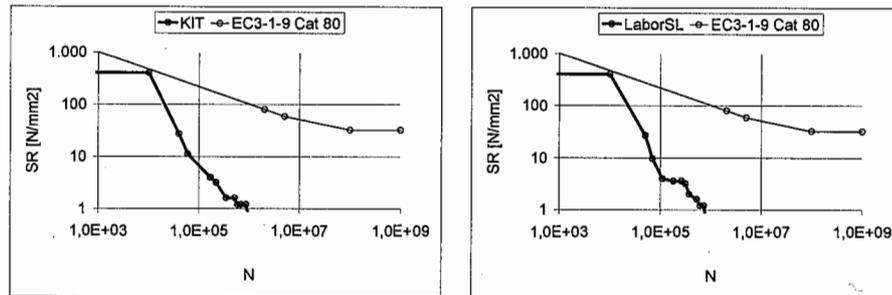
Fig. 3. Most unfavourable scenario for a fatigue test with the amplitude spectra given in fig. 2; left: KIT; right: LaborSL
