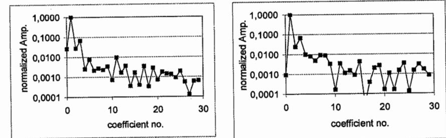
Fig. 2. Normalized amplitude spectrum of the curves in fig. 1; logarithmic scale; left: KIT; right: LaborSL
