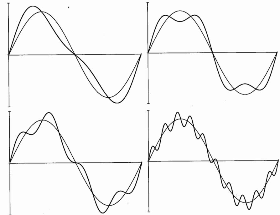
Fig. 4. Degraded sinusoidal shapes which produce 5 % damage additional to the first harmonic; the normalized size of the second amplitude is given in brackets top left: 1. + 2. harmonic (0,293); top right: 1. + 3. harmonic (0,256); bottom left: 1. + 4. harmonic (0,232); bottom right 1. + 10. harmonic (0,171);
