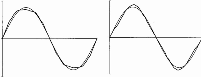
Fig. 1. Degraded sinusoidal response in fatigue test, represented by a 30-term Fourier sum
